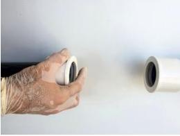
5. Coat O-Rings with silicone lube. Place the O-Rings into their channels on the flow cell and tighten the barrel nuts.
