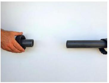
4. Coat the pipe and union collars with PVC primer and glue. Slide collars over the pipe and hold in place until a solid connection is made. Please wait a minimum of 10 minutes to allow the glue to cure.
